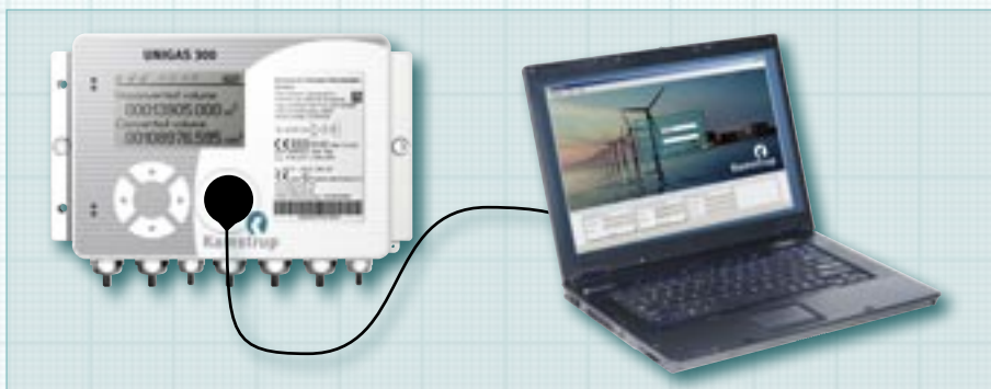
Local configuration of UNIGAS 300 with UNITOOL
